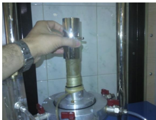
(a) assembling of the specimen on the cell base
