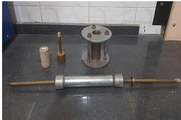
Fig. 2. The Harvard miniature compaction apparatus and a compacted sample.
