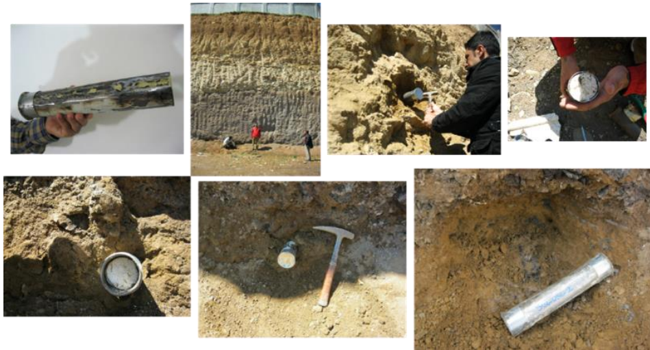
Fig. 2. Implantation of suitable metal pipes in river sediments (sandy lens) to determine OSL age
